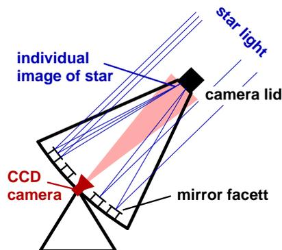
**Fig. 1.** Mirror alignment technique. The alignment of the mirror facets is done by using images of stars. Individual light spots in the focal plane (camera lid) are imaged with a CCD camera for optical feedback.
