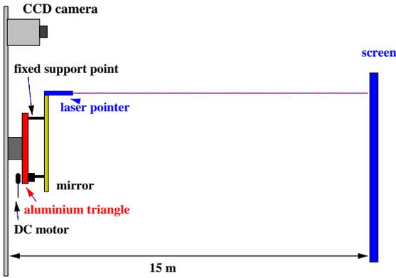
**Fig. 3.** Test setup for the test of the complete mirror support drive system
