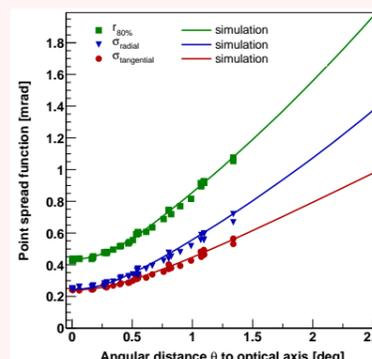
**Off-axis behaviour of the point spread function.** The measurements are in excellent agreement with simulations.
