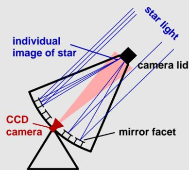
**Mirror alignment technique:** The telescope is pointed towards an appropriate star whereupon all mirror facets generate individual images of the alignment star in the focal plane. Actuator movements change the location of the corresponding image which is observed by a CCD camera.
