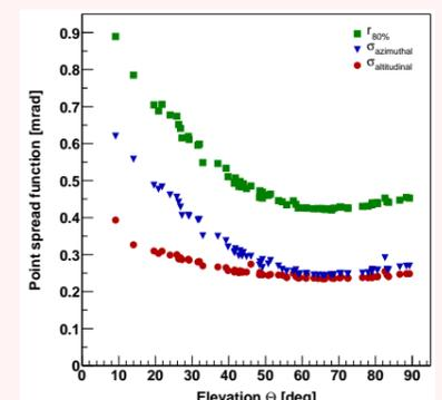
**Point spread function with varying elevation.** The curves are nearly flat in the usual working range between 45° and 90° elevation, indicating a good stability of the support structure.
