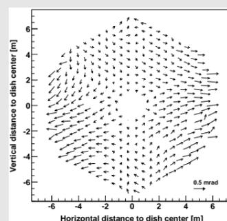
CCD images of spot matrix at different elevations → relative movement of spots → deflection of mirror facets → deformation of dish structure.
