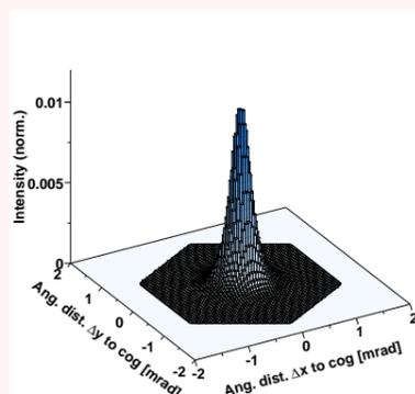
**Intensity distribution in the focal plane** of an imaged star in comparison with the hexagonal shape of a pixel of the PMT Cherenkov camera. The complete amount of light is well within one pixel.
