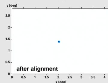
Light spots before and after the mirror alignment as seen by the CCD camera (log. scale).
