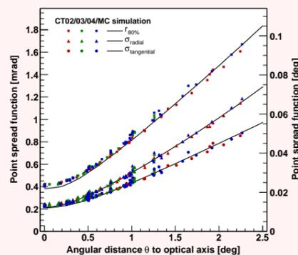
**Off-axis behaviour of the point spread function. The measurements are in good agreement with Monte Carlo simulations.**
