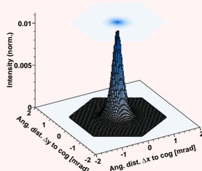
**On-axis intensity distribution of a star on the camera lid after alignment (CT04).** The hexagonal border indicates the size of a pixel of the PMT Cherenkov camera. **The complete amount of light is well within one pixel.**
