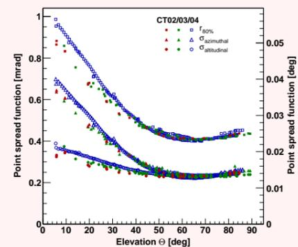
**Point spread function with varying elevation.** The curves are nearly flat in the usual working range (45°–90°), indicating a **good stability of the support structure**. In addition, **all reflectors behave very similar**.
