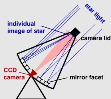
**Mirror alignment technique:** The telescope is pointed towards an appropriate star whereupon all mirror facets generate individual images of the alignment star in the focal plane (closed lid of the PMT camera). Actuator movements change the location of the corresponding image which is observed by a CCD camera.
