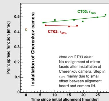
**Evolution of the point spread function at 65° elevation.** Only a small increase of 0.022 mrad or 6% per year for  $r_{80\%}$  is observed (CT03, the first telescope), indicating an outstanding long-term stability of the telescope structure.
