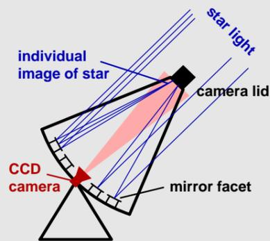
**Mirror alignment technique:** The telescope is pointed towards an appropriate star whereupon all mirror facets generate individual images of the alignment star in the focal plane (closed lid of the Cherenkov camera). Actuator movements change the location of the corresponding image which is observed by a CCD camera at the center of the dish.
