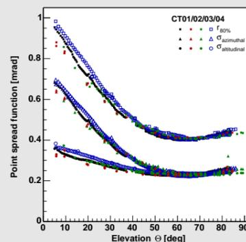
**Effect of the elevation-dependent deformation on the PSF.** The curves are nearly flat in the usual working range (45°–90°), indicating a good stability of the support structure. In addition, all reflectors behave very similar.
