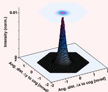
**Left: On-axis intensity distribution of a star image on the lid (CT04).** The hexagonal border indicates the size of a photomultiplier pixel.
