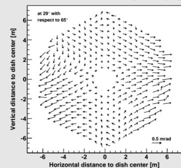
**Mirror deflections at 29° elevation with respect to 65° (CT03, scaled by  $\sqrt{\text{deflection}}$ ).**
