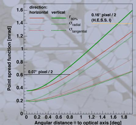
Left: Simulated point spread function as a function of the angular distance to the optical axis. The lower curves (n) show the scenario in which every mirror facet is manufactured to have its nominal focal length. The top curves (1) represent the case in which all facets are manufactured to have an identical focal length. A difference between these two cases is hardly seen. Curves are shown for the vertical direction only.
