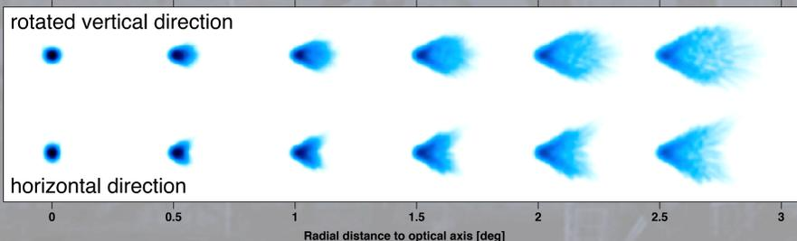
Simulated point spread function of the H.E.S.S. II reflector for various angular distances to the optical axis. The top series of spot shapes represent the (rotated) development along the vertical direction; the bottom series are for the horizontal direction. The intensity scale is logarithmic. Note that the actual active field of view is limited to a radius of 1.6 degrees.
