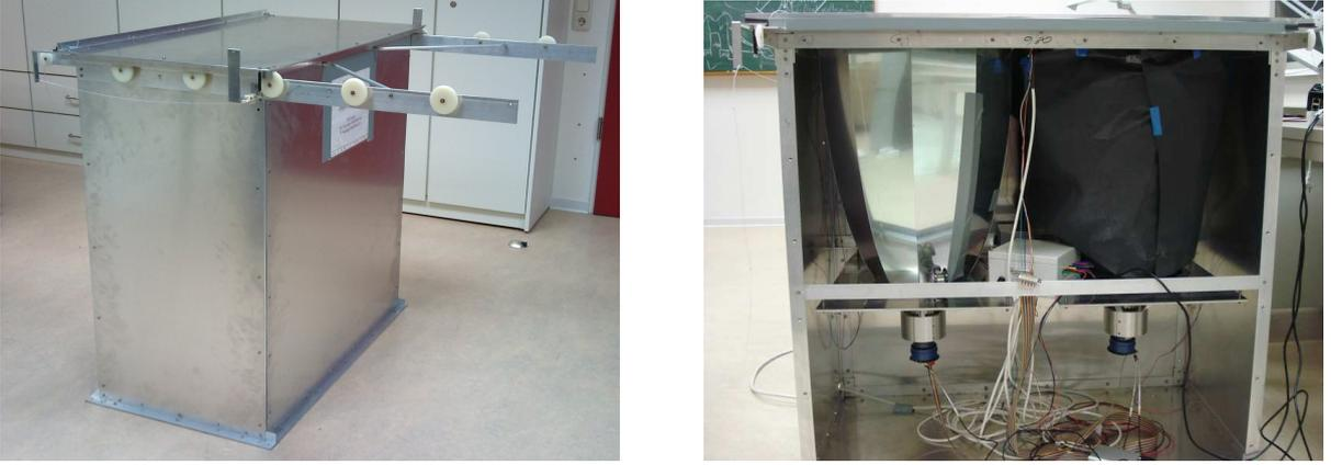
Figure 4.4: The second prototype for a H<sub>i</sub>SCORE detector station. The left picture shows the station from outside, including the lid mounting. The right picture shows the inside of the station with the two Winston cones (the right cone is temporarily shielded with black paper for tests) and the PMTs.
