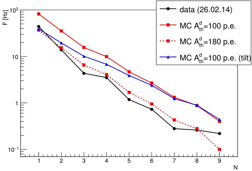
FIGURE 6.5: Detector multiplicity of the 9-station array as a function of the number of triggered stations. The data from 26.02.14 is shown for comparison.
