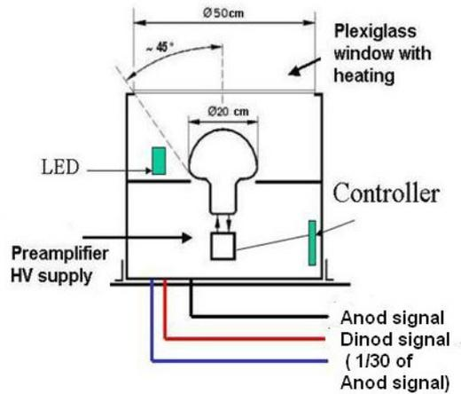
FIGURE 4.1: Optical detector.
