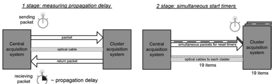
FIGURE 4.3: Concept of the time synchronization system [63].
