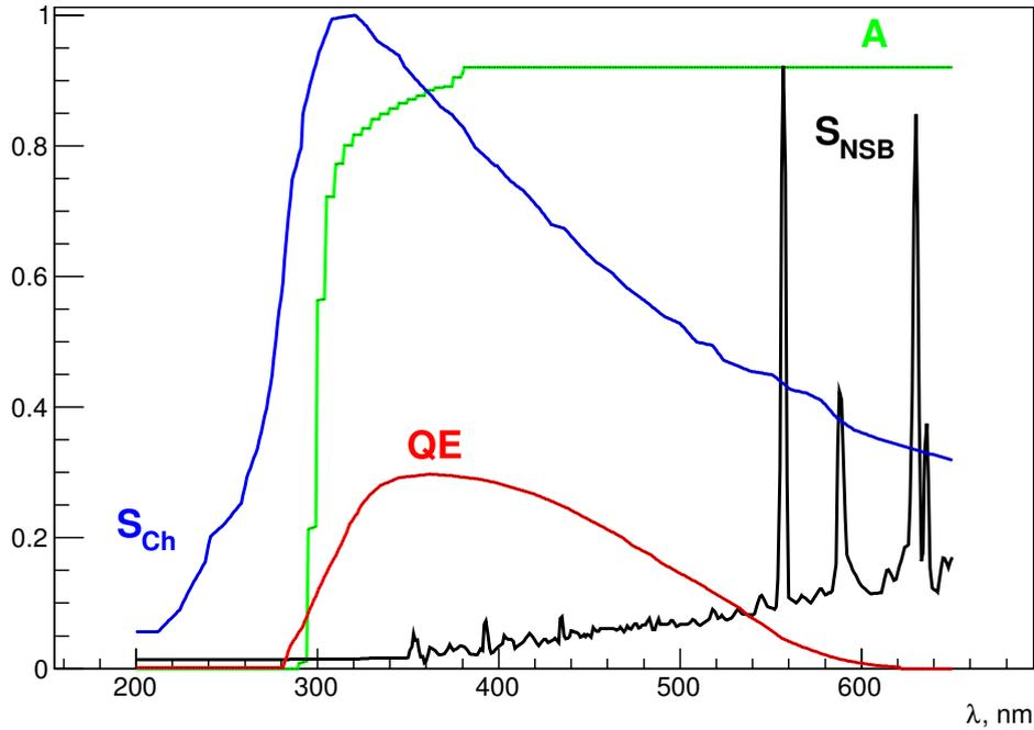
FIGURE 5.9: Quantum efficiency  $QE(\lambda)$  of the 9352KB photomultiplier as a function of wavelength of the incident light.  $A(\lambda)$  represents the acrylic glass transmission. The spectrum of the night sky  $S_{\text{NSB}}(\lambda)$  and the attenuated Cherenkov spectrum  $S_{\text{Ch}}(\lambda)$  are shown as well.
