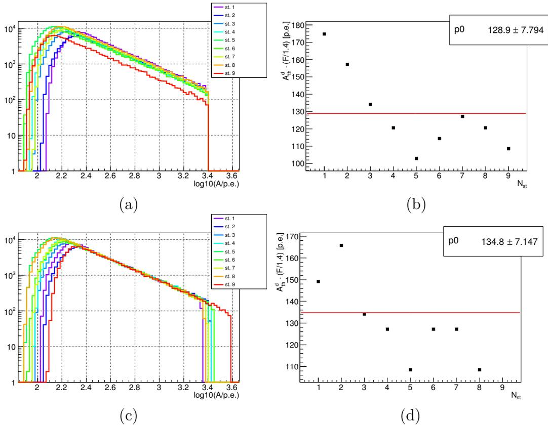
FIGURE 5.14: Raw integral spectra of sum-channels calibrated from units of the DAQ-2 to photoelectrons (*left*) and average discriminator thresholds  $A_{th}^d$  for nine stations (*right*). (a, b) Spectra after applying the common conversion factor  $C=2.5$  p.e./a.u. (c, d) Spectra after applying the same conversion factor  $C$  and the additional relative calibration. Station threshold is defined at the level of 1/2 from the maximum of the spectrum.
