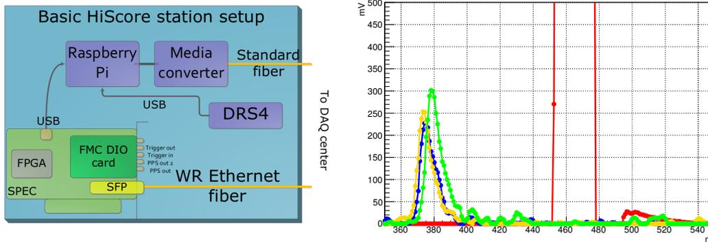
FIGURE 5.5: *Left:* The basic White Rabbit setup [81] WR-node (SPEC card) with WR-fiber, Raspberry Pi and DRS4 evaluation board. *Right:* Three anode pulses (1 ns step) and the WR strobe recorded by the DRS4 evaluation board.
