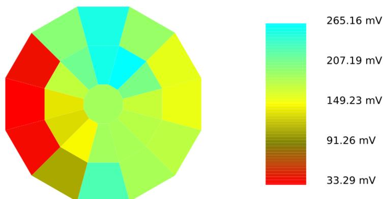
FIGURE 5.6: Photocathode uniformity of the R5912 multiplier [83].
