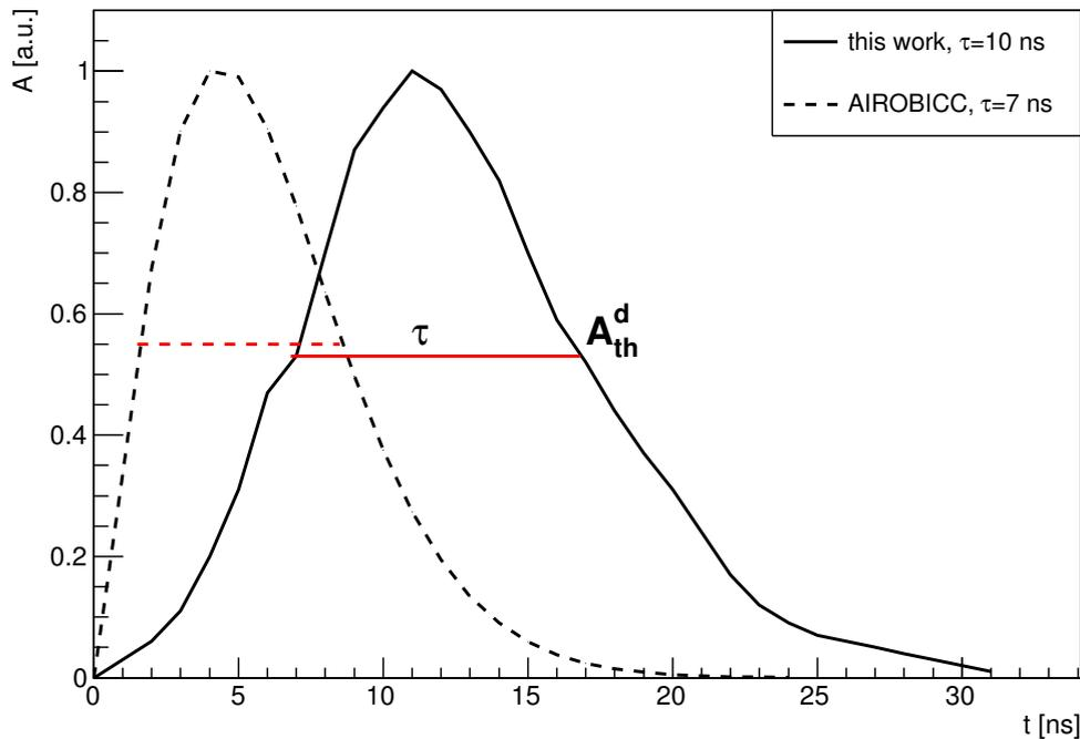
FIGURE 5.11: The HiSCORE detector response. Signal shape was measured with the oscilloscope using a fast LED source. The AIROBICC response [89] is shown as well.
