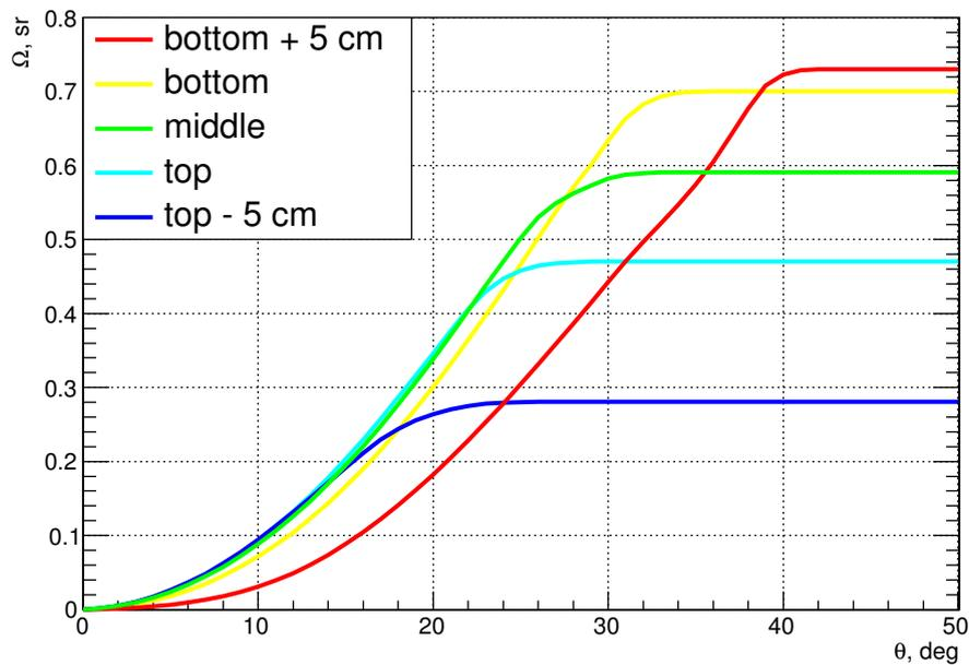
FIGURE 5.7: Angular and cumulative acceptance of the Winston cone for various PMT positions.
