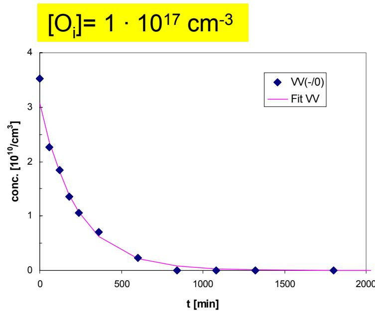
Time dependence of  $V_2$  concentration in DOFZ-diodes during annealing at 250°C.
