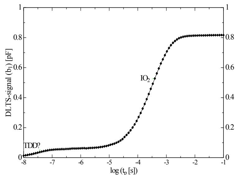
Direct measurement of capture cross-section for electrons at 60K
