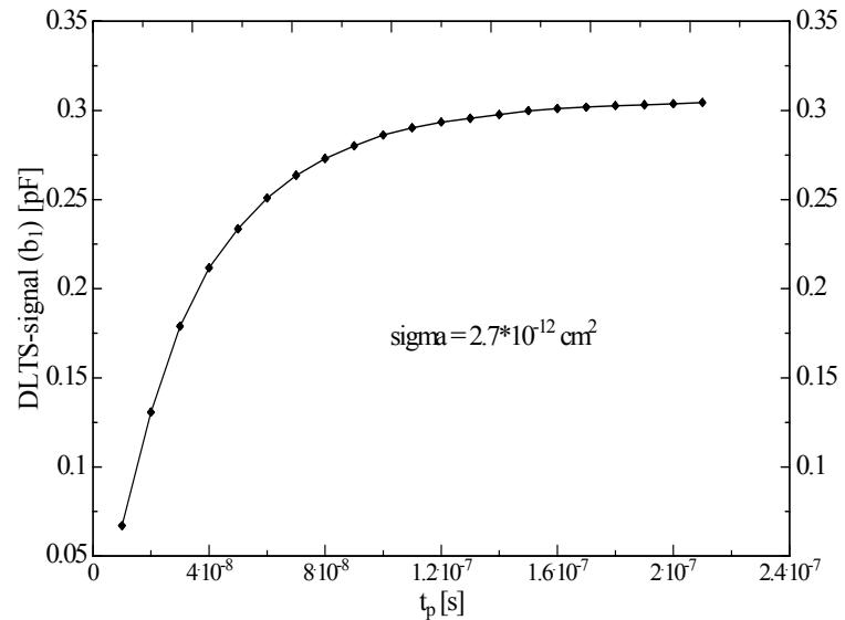
Direct measurement of the TDD electron capture cross-section performed at 60K.
