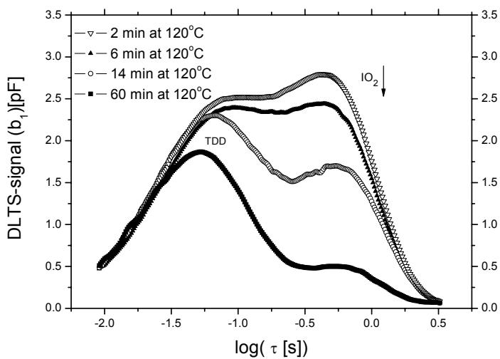
High-resolution DLTS spectra performed at 62K during - isothermal annealing at 120°C
