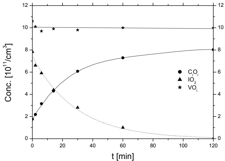
Isothermal annealing at  $120^\circ\text{C}$
